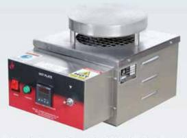
Supplied complete with pilot indicating lamps for MAINS and HEATER operation, power plug and 2 meter long cord wire to work on 220/230 AC, Single phase.
